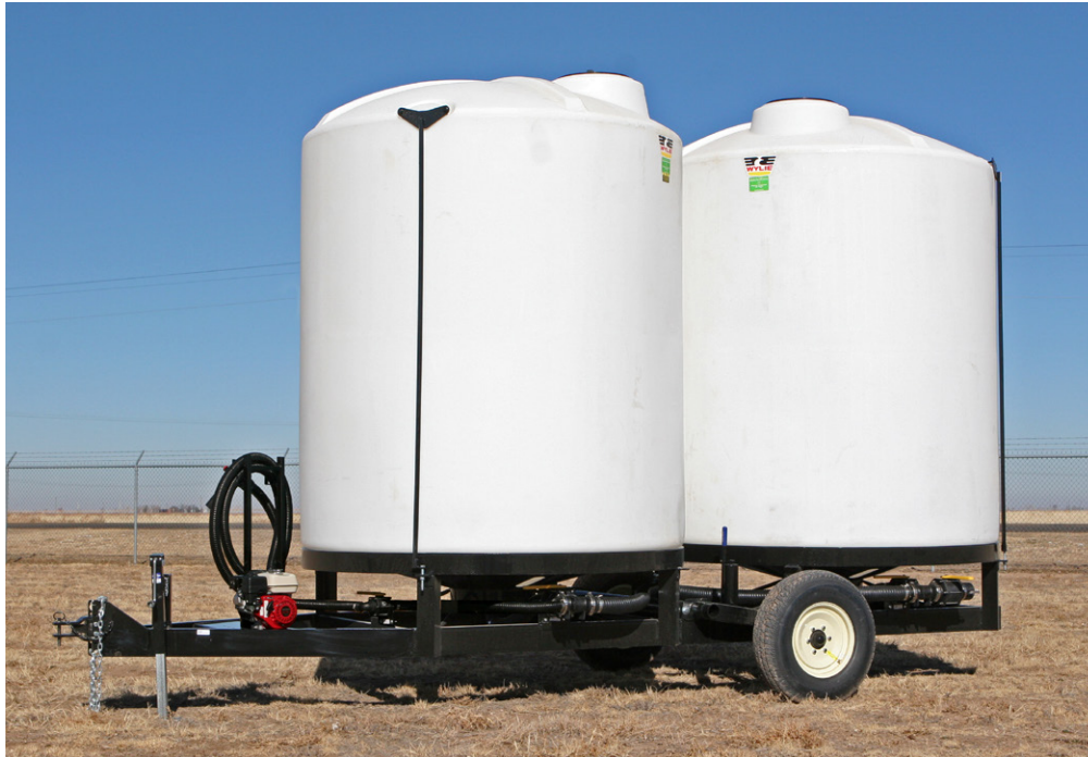
Double cone trailer offers 6,000 gallons total capacity of portable storage
