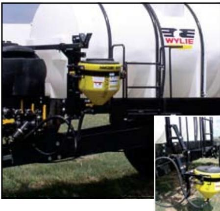
*Safety and ease of operation are key to the design of the 1600. A 100 gallon fresh water tank has a valve for hand washing or can be used to flush the spraying system. The opaque tank prevents algae growth.*
