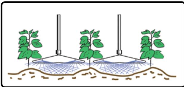
**Back View** – Spray is directed across the weeds while the shield protects the crop foliage. No need to worry about crop damage with the low-profile aluminum shield...even during those mid to late season applications.
