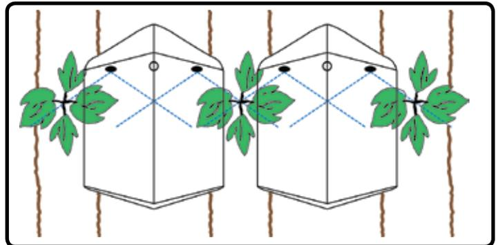
**Top View** – Dual 110° broadcast nozzles under each shield cover the weeds from row to row.
