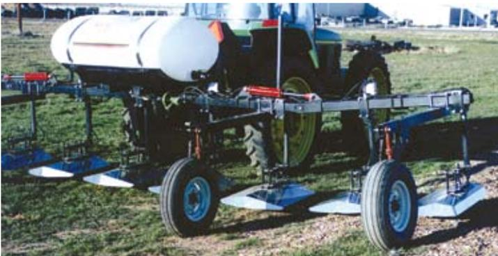
*Folding Spray Shield wing flexes 10° for more versatility on terraces and uneven ground.*
