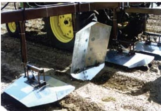
*Shields rotate when obstructions are hit.
